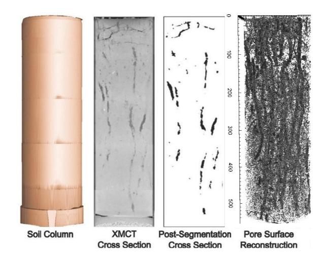
Using morphological operators, labeling and masking
